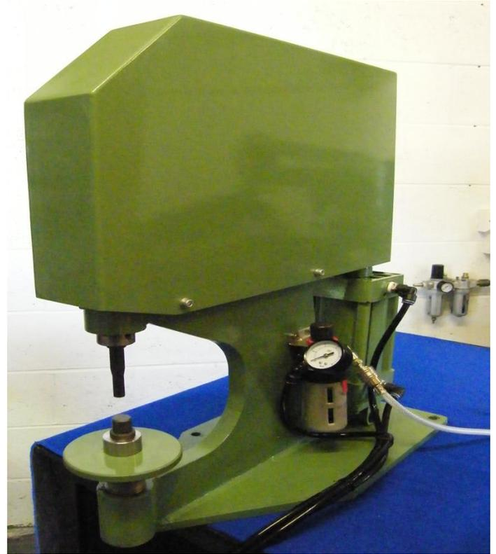
The pneumatic cylinder mounted at the rear of the head is connected to the downward moving punch holder by a simple leverage system, giving a riveting stroke of 20mm. The foot pedal can be located from either left or right foot operation.
